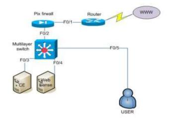
Fig. 7 The data center core layer
