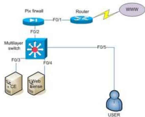
Fig. 3 The data center core layer
