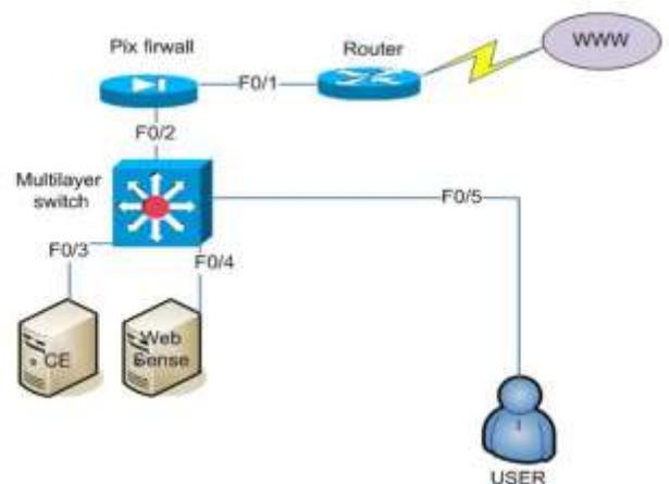
Fig. 7 The data center core layer
