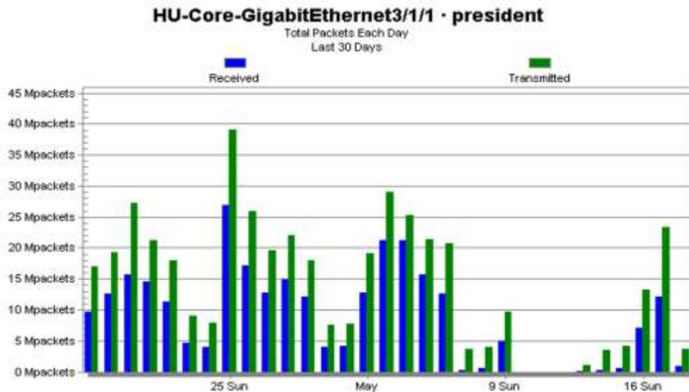
Fig. 10 The transmit (upload) over president building interface and the receives (download) packets for 30 days
