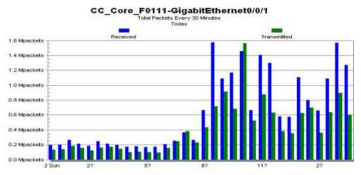
Fig.5 The received (upload) over the main interface compared to transmitted (download) packets
