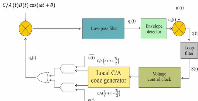
Fig. 3. A tracking loop with trembling tau [15]
