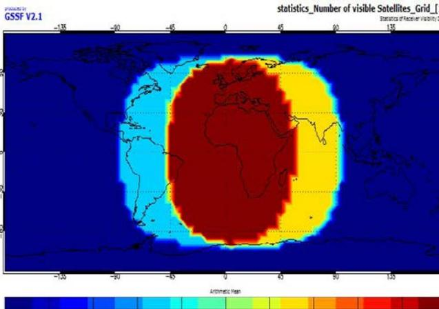
Fig. 7. Visibility of SBAS system satellites
