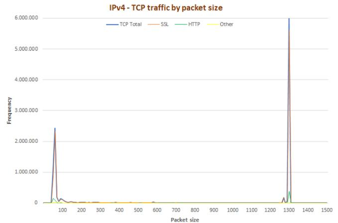
Fig. 5. IPv4 – TCP applications traffic classified by length
