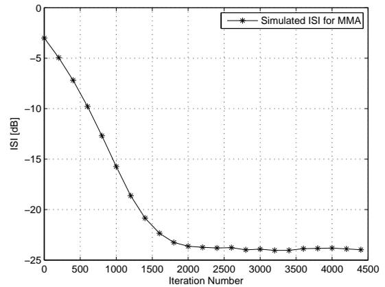
Fig. 11. ISI as a function of iteration number for a 16QAM source input going through channel3. The averaged results were obtained in 100 Monte Carlo trials for a SNR=30 dB.  $\mu_{MMA} = 0.00004$ .
