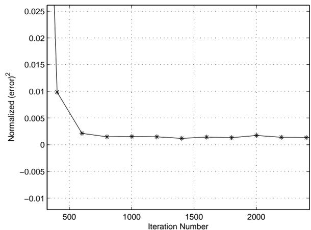
Fig. 7. Normalized zoomed in version for the  $err(5)$  as a function of iteration number for a 16QAM source input going through channel1. The averaged results were obtained in 100 Monte Carlo trials for a SNR=20 dB.  $\mu_{MMA} = 0.0001$ .
