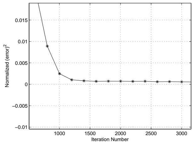
Fig. 13. Normalized zoomed in version for the  $err(5)$  as a function of iteration number for a 16QAM source input going through channel3. The averaged results were obtained in 100 Monte Carlo trials for a SNR=30 dB.  $\mu_{MMA} = 0.00004$ .
