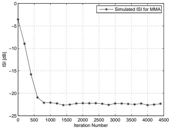
Fig. 2. ISI as a function of iteration number for a 16QAM source input going through channel1. The averaged results were obtained in 100 Monte Carlo trials for a SNR=30 dB.  $\mu_{MMA} = 0.0001$ .
