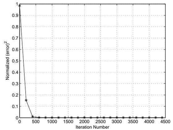
Fig. 6. Normalized  $err(5)$  as a function of iteration number for a 16QAM source input going through channel1. The averaged results were obtained in 100 Monte Carlo trials for a SNR=20 dB.  $\mu_{MMA} = 0.0001$ .
