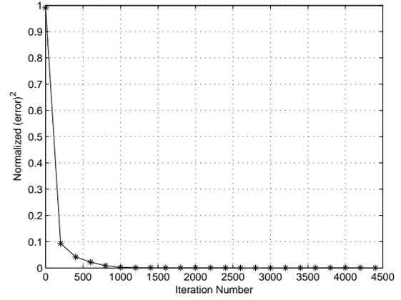
Fig. 12. Normalized  $err(5)$  as a function of iteration number for a 16QAM source input going through channel3. The averaged results were obtained in 100 Monte Carlo trials for a SNR=30 dB.  $\mu_{MMA} = 0.00004$ .
