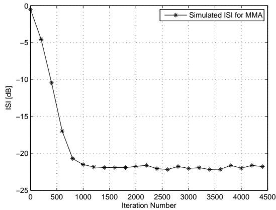
Fig. 8. ISI as a function of iteration number for a 16QAM source input going through channel2. The averaged results were obtained in 100 Monte Carlo trials for a SNR=30 dB.  $\mu_{MMA} = 0.0001$ .
