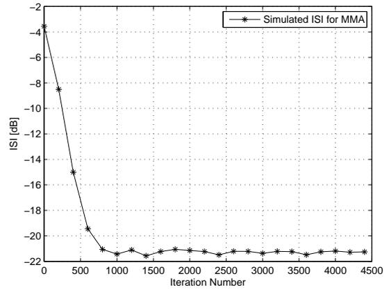
Fig. 5. ISI as a function of iteration number for a 16QAM source input going through channel1. The averaged results were obtained in 100 Monte Carlo trials for a SNR=20 dB.  $\mu_{MMA} = 0.0001$ .
