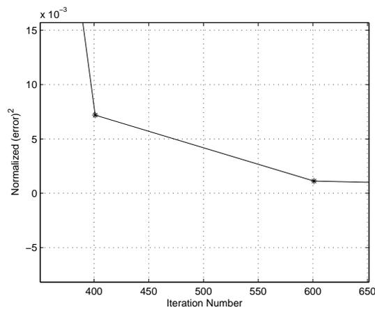
Fig. 4. Normalized zoomed in version for the  $err(5)$  as a function of iteration number for a 16QAM source input going through channel1. The averaged results were obtained in 100 Monte Carlo trials for a SNR=30 dB.  $\mu_{MMA} = 0.0001$ .
