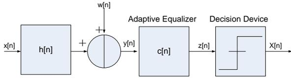
Fig. 1. Block diagram of a baseband communication system.
