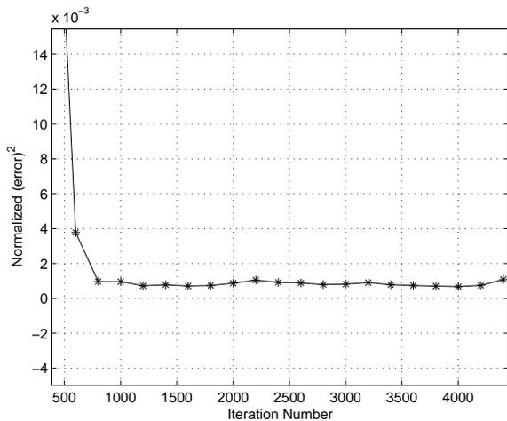
Fig. 10. Normalized zoomed in version for the  $err(5)$  as a function of iteration number for a 16QAM source input going through channel2. The averaged results were obtained in 100 Monte Carlo trials for a SNR=30 dB.  $\mu_{MMA} = 0.0001$ .
