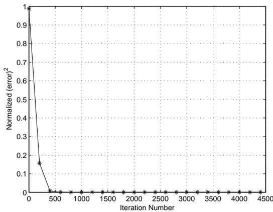
Fig. 3. Normalized  $err(5)$  as a function of iteration number for a 16QAM source input going through channel1. The averaged results were obtained in 100 Monte Carlo trials for a SNR=30 dB.  $\mu_{MMA} = 0.0001$ .
