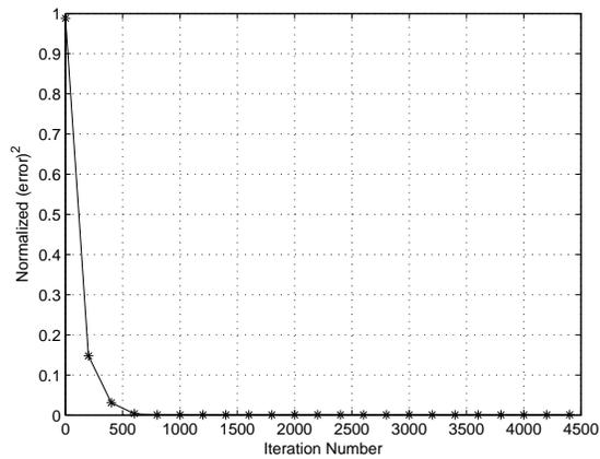
Fig. 9. Normalized  $err(5)$  as a function of iteration number for a 16QAM source input going through channel2. The averaged results were obtained in 100 Monte Carlo trials for a SNR=30 dB.  $\mu_{MMA} = 0.0001$ .
