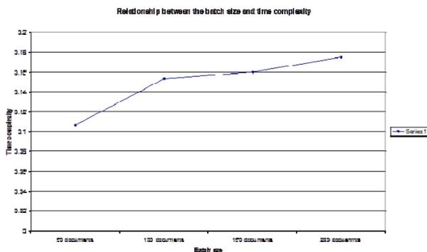
Fig. 9 Relationship between the batch size and the time complexity of the classification phase
