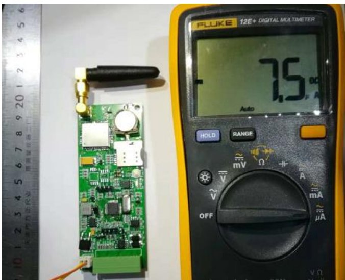
Fig. 8. The NB-IoT-based RTU running in an ultra-low-power consumption mode (with a quiescent current of 7.5 \mu A).
