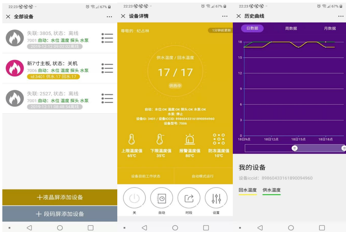
Fig. 16. Screenshots of the developed Android mobile application for the smart electric boiler control system.
