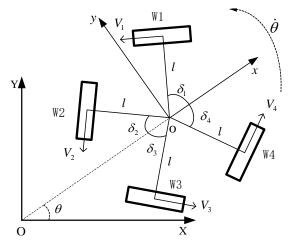
Fig. 1. Wheel placement of mobile robot
