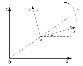
Fig. 2. The motion relationship of mobile robot
