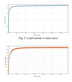
Fig. 6. PFC output voltage vs time curve
