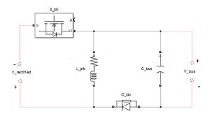
Fig. 3. Buck-boost converter
