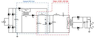
Fig. 2.3. Circuit of LED driver based on Flyback and Class – E converter [24]
