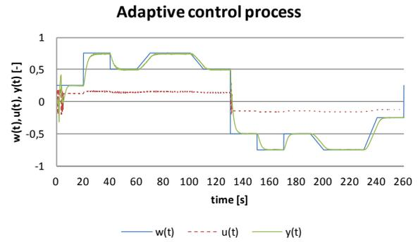
Fig. 33 Multi-level control process with using of the Hammerstein and Wiener models for  $T_0 = 0.125s$
