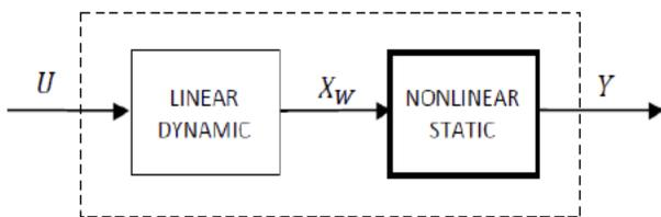
Fig. 2 Wiener model of the nonlinear system [6]
