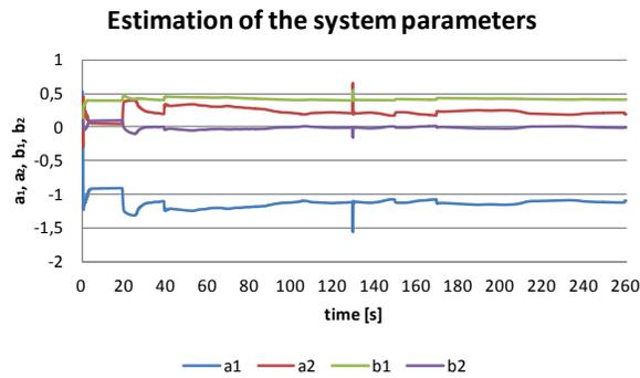
Fig. 32 Estimation of system parameters for  $T_0 = 0.125s$
