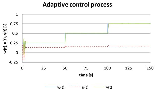
Fig. 29 Control process with using of the Hammerstein and Wiener models for  $T_0 = 0.15s$
