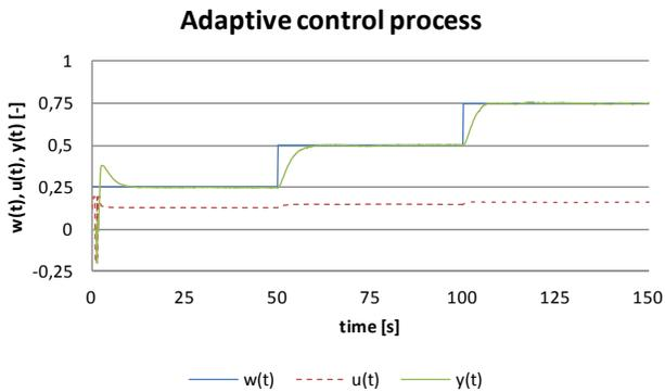
Fig. 17 Control process with using of the Hammerstein and Wiener models for  $T_0 = 0.15s$
