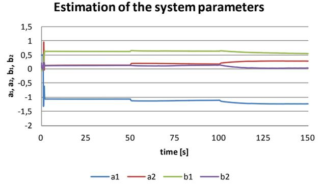
Fig. 28 Estimation of system parameters for  $T_0 = 0.125s$
