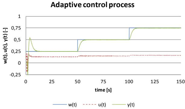
Fig. 15 Control process with using of the Hammerstein and Wiener models for  $T_0 = 0.125s$
