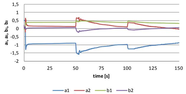
Fig. 24 Estimation of system parameters for  $T_0 = 0.125s$
