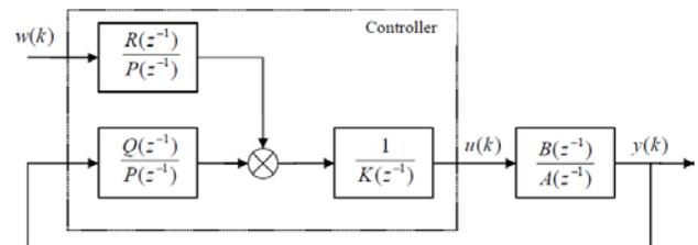
Fig. 5 2DOF control system configuration [5]
