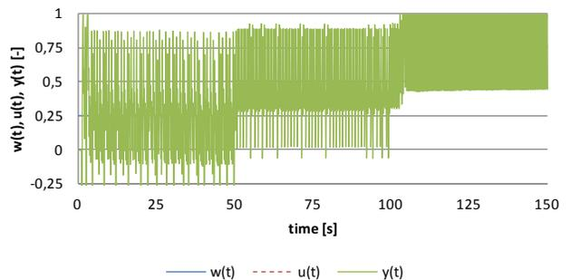
Fig. 19 Control process without control action limitation for  $T_0 = 0.125s$
