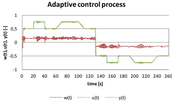
Fig. 31 Multi-level control process with control action limitation for  $T_0 = 0.125s$
