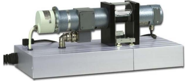
Fig. 4 Nonlinear system – the servo-speed mechanism AMIRA DR300
