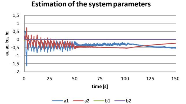
Fig. 8 Estimation of system parameters for  $T_0 = 0.125s$
