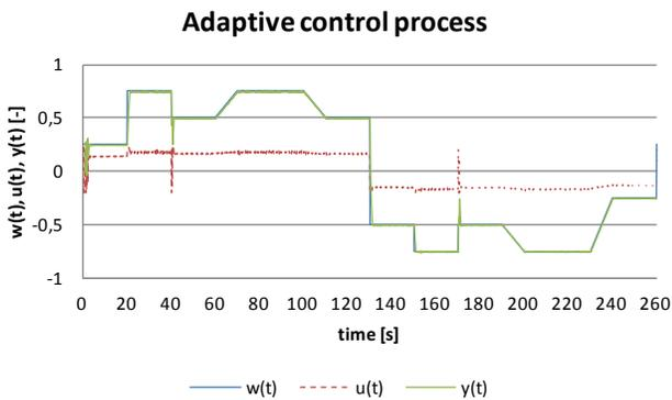
Fig. 37 Multi-level control process with using of the Hammerstein and Wiener models for  $T_0 = 0.125s$
