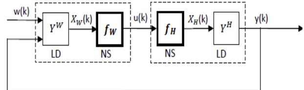
Fig. 3 Closed control loop with the controlled system of the Hammerstein type and the controller of the Wiener type.
