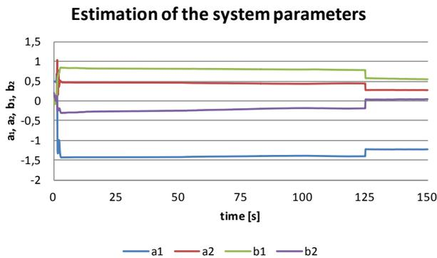
Fig. 16 Estimation of system parameters for  $T_0 = 0.125s$
