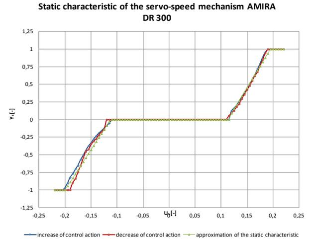
Fig. 6 Static characteristic of the nonlinear system AMIRA DR300
