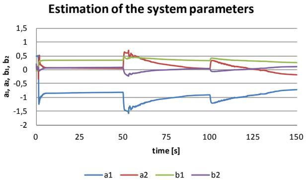
Fig. 12 Estimation of system parameters for  $T_0 = 0.125s$
