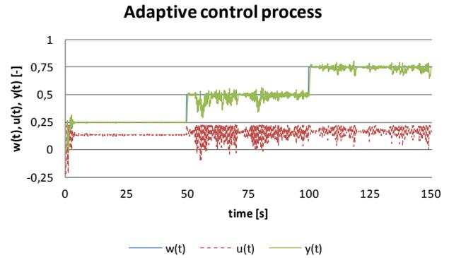
Fig. 13 Control process with control action limitation for  $T_0 = 0.15s$
