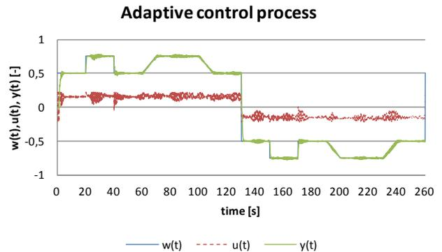
Fig. 35 Multi-level control process with control action limitation for  $T_0 = 0.125s$
