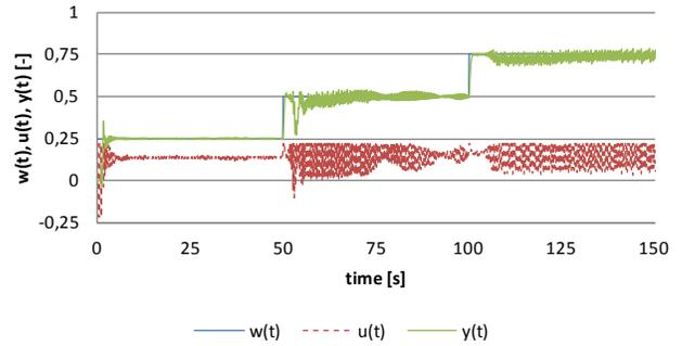
Fig. 23 Control process with control action limitation for  $T_0 = 0.125s$
