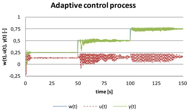
Fig. 11 Control process with control action limitation for  $T_0 = 0.125s$
