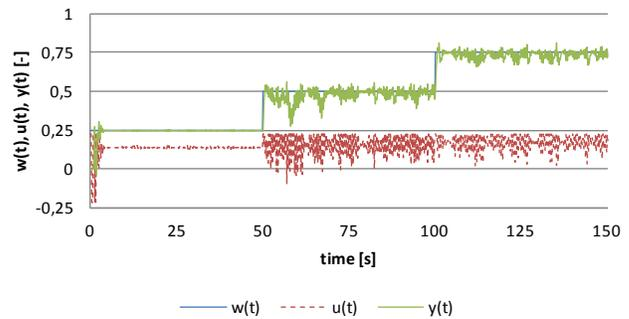
Fig. 25 Control process with control action limitation for  $T_0 = 0.15s$
