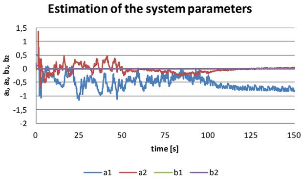
Fig. 10 Estimation of system parameters for  $T_0 = 0.15s$
