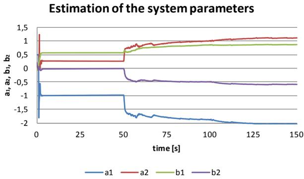
Fig. 26 Estimation of system parameters for  $T_0 = 0.15s$
