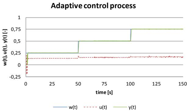
Fig. 27 Control process with using of the Hammerstein and Wiener models for  $T_0 = 0.125s$
