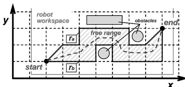
Fig. 1 Free range for possible robot movement
