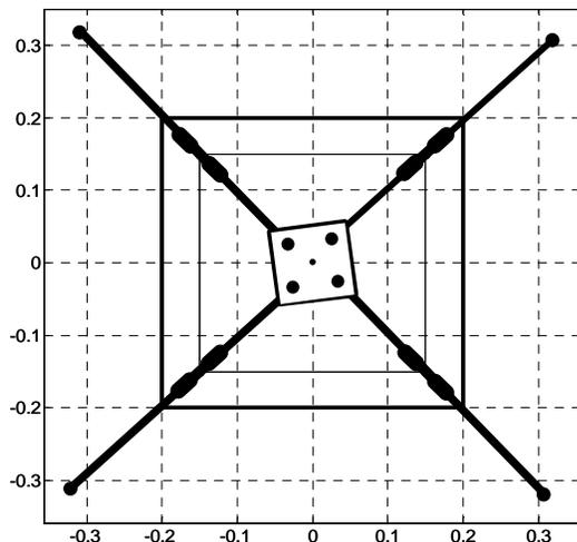
Fig. 6 Scheme: 4RPR parallel robot 'Moving Slide'
