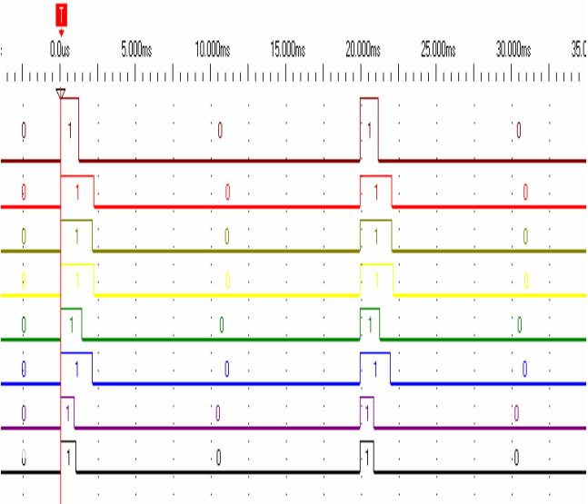
Fig. 14 50 Hz PWM output with  $12.5 \mu s$  time base
