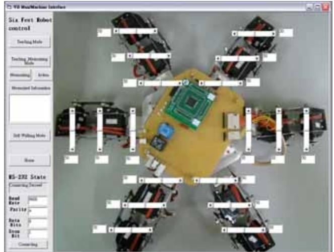
Fig. 19 Man machine interface windows
