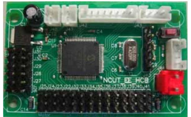
Fig. 12 photo of Control PCB
