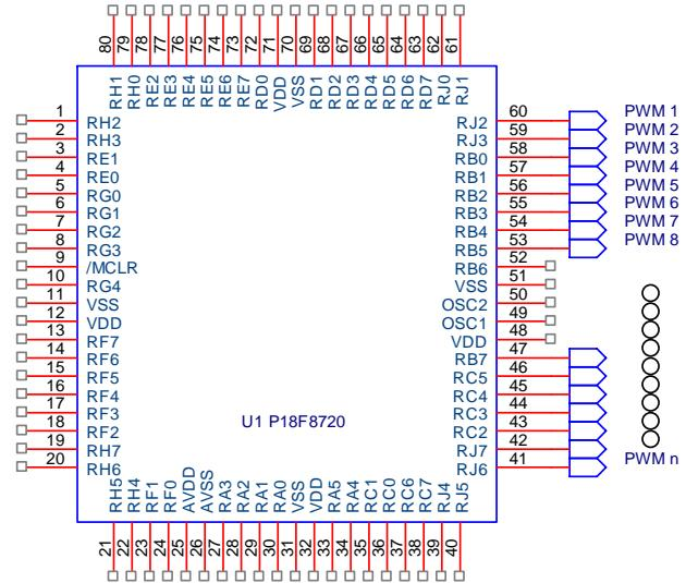
Fig. 3 Schematic diagram of microcontroller based PWM signal generation scheme
