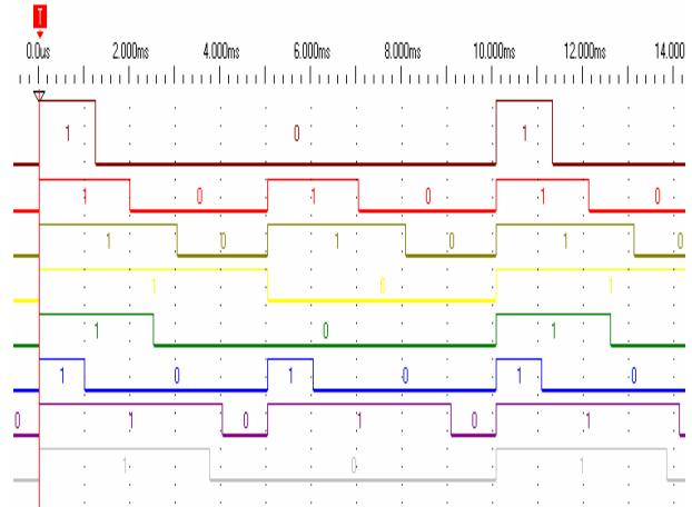
Fig. 7 Hybrid PWM signals
