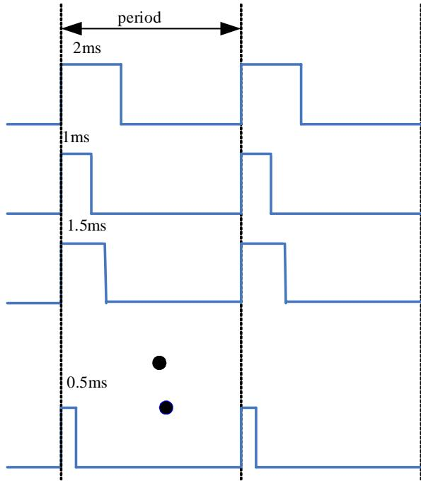
Fig. 2 Desired synchronized multi-channel PWM signals
