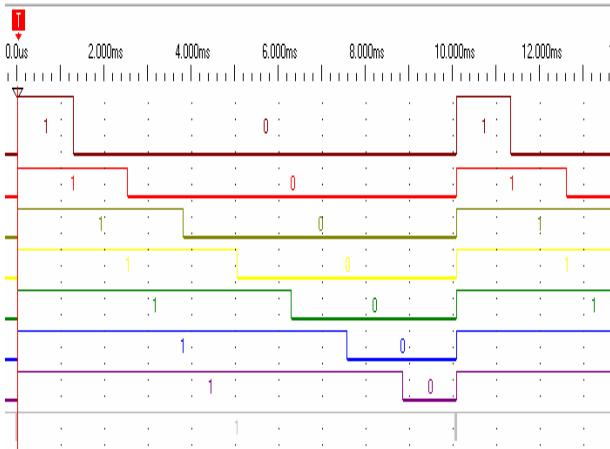
Fig. 6 18 channels 100Hz PWM signals output
