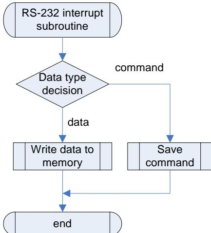
Fig. 21(b) RS-232 interrupt subroutine flowchart of PIC microcontroller
