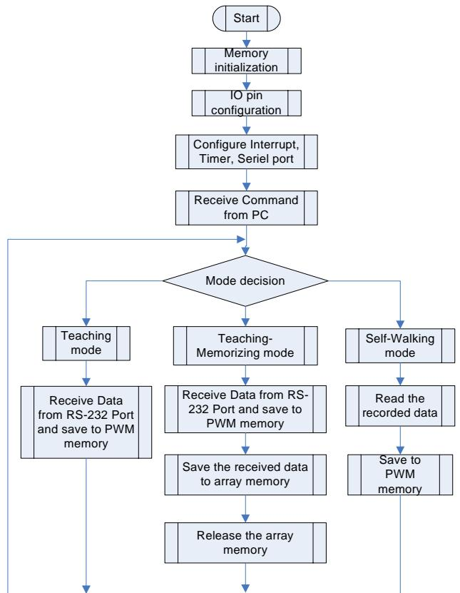
Fig. 21(a) Main program flowchart of PIC microcontroller
