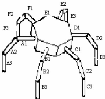
Fig. 16 Motor number of each joint
