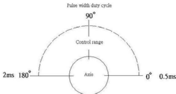
Fig. 9 Relationship of pulse width and axis output of RC motor
