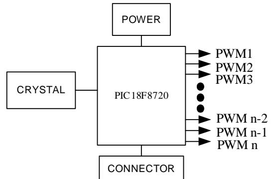
Fig. 11 Block diagram of control PCB
