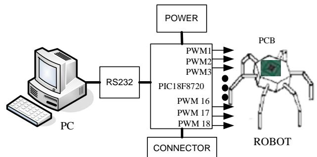
Fig. 18 Schematic diagram of man-machine interface system
