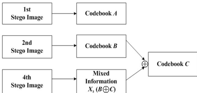
Fig. 7 the reconstruction of the three VQ codebooks when receiving the first, second, and fourth stego images
