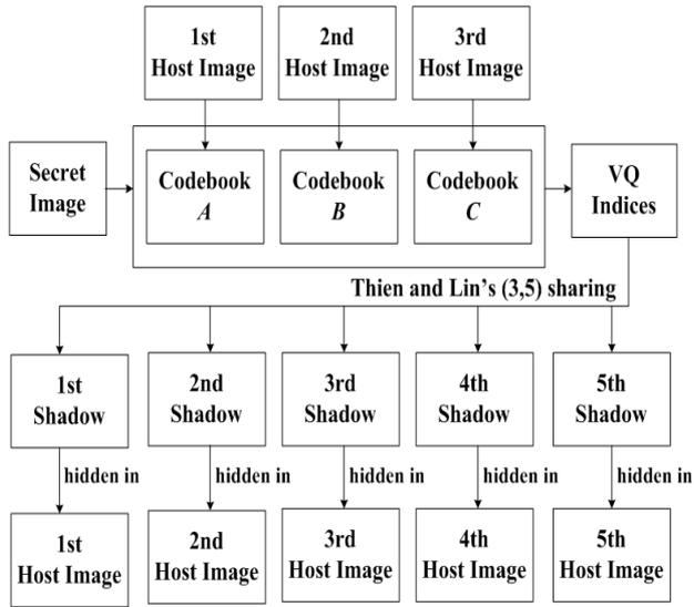
Fig. 5 the flow of the generation, sharing, and hiding of the VQ indices
