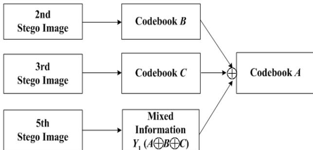
Fig. 8 the reconstruction of the three VQ codebooks when receiving the second, third, and fifth stego images
