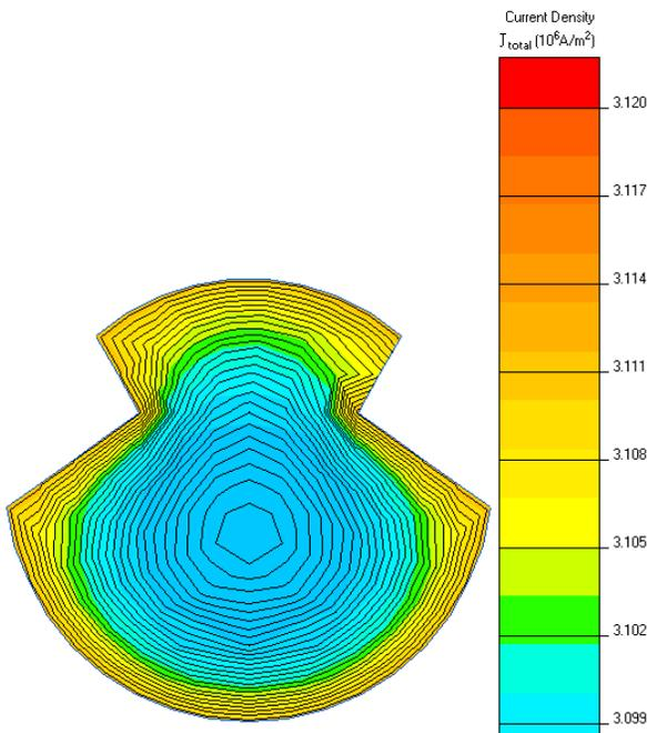
Fig. 11. The current density distributions – AC current,  $i=301A$
