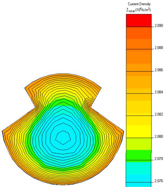
Fig. 10. The current density distributions – AC current,  $i=201A$
