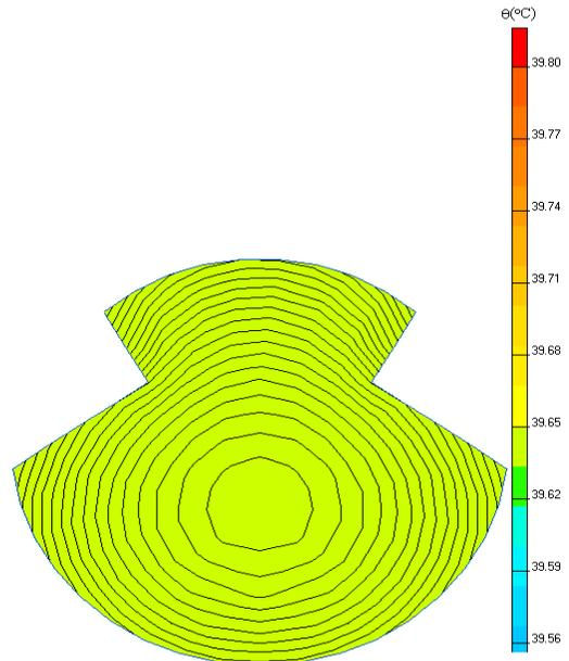
Fig. 12. Temperature in contact wire –AC current ,  $i=201A$ ,  $\theta_0=22.7^{\circ}C$
