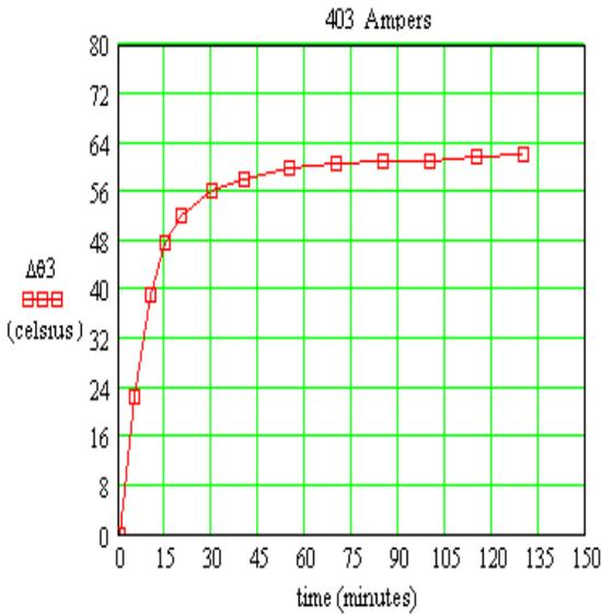
Fig.19 Contact wire temperature evolution for 403 amperes, A.C. current
