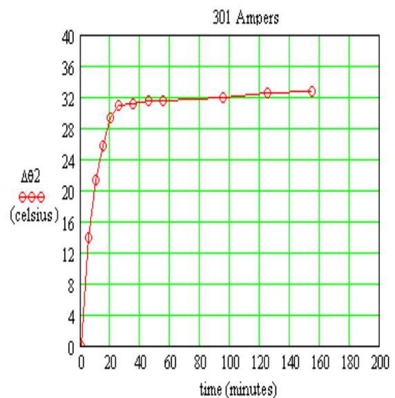
Fig.18 Contact wire temperature evolution for 301 amperes, A.C. current
