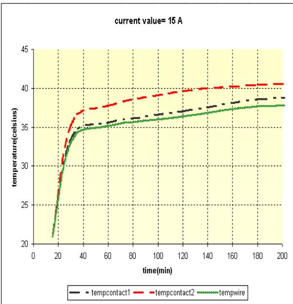
Fig. 20 Measured temperatures in contact for 15 A, AC current
