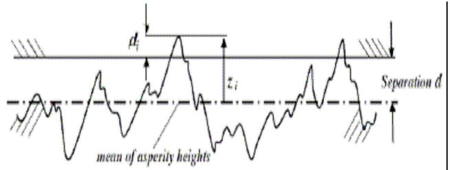
Fig.8 Contact between rough surfaces modeled as contact between a rough surface and a smooth surface
