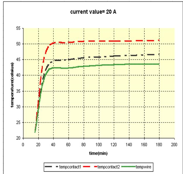
Fig. 21 Measured temperatures in contact for 20 A, AC current
