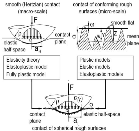
Fig.6 Mechanical problem overview for spherical rough surfaces
