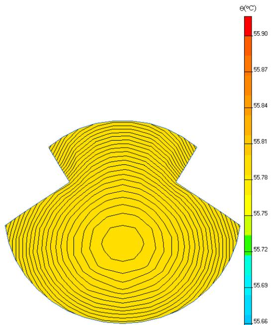
Fig. 13. Temperature in contact wire –AC current ,  $i=301A$ ,  $\theta_0=23.5^{\circ}C$
