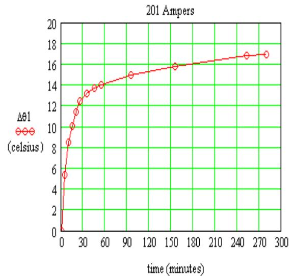
Fig.17 Contact wire temperature evolution for 201 amperes, A.C. current
