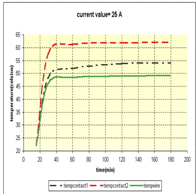
Fig. 22 Measured temperatures in contact for 25 A, AC current
