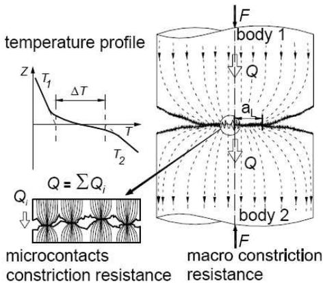
Fig.7 Non-conforming rough contact
