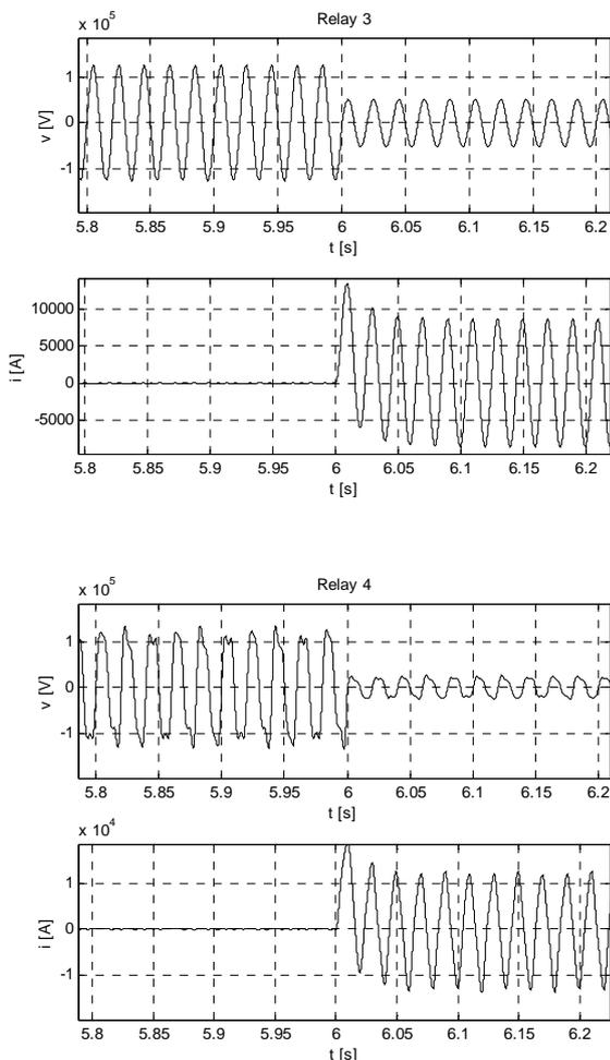
Fig. 2 voltage and current signals as observed by the  $R_3$  and  $R_4$  relays involved in the line trip
