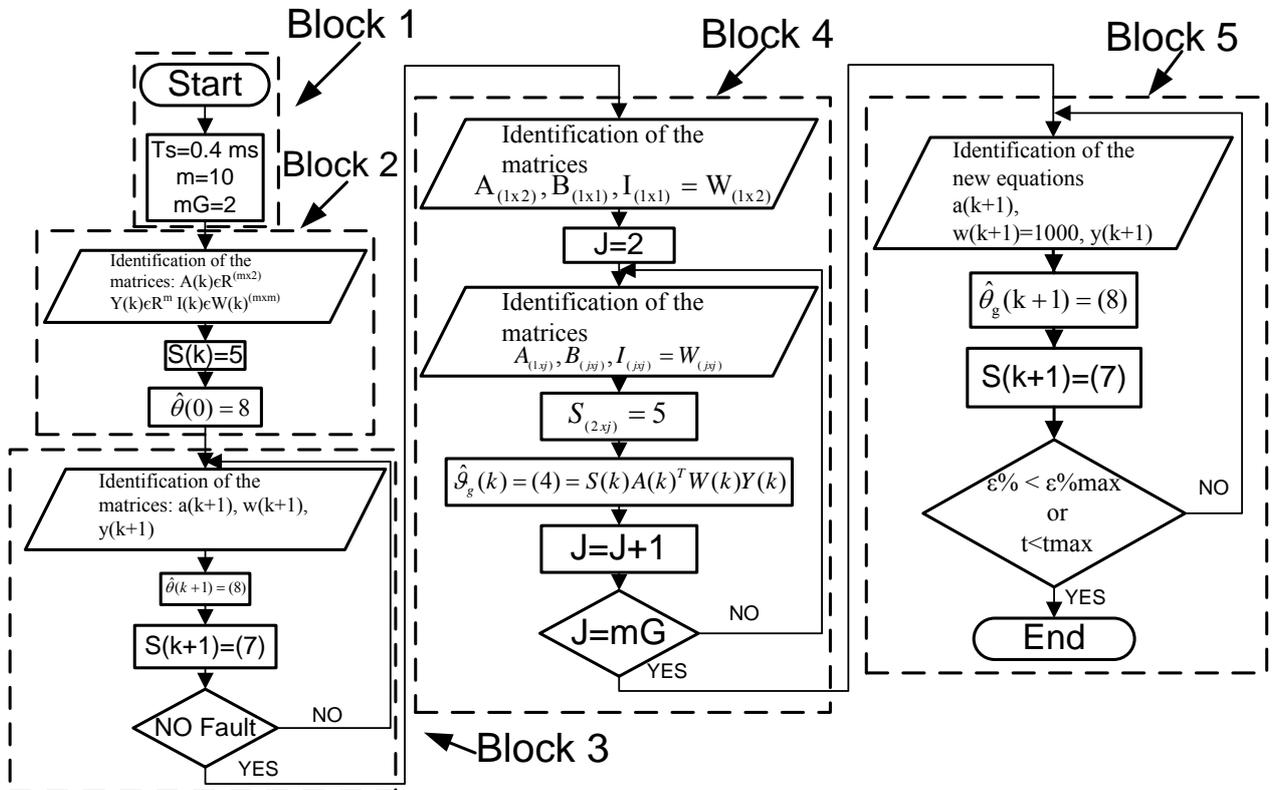
Fig. 1 the implemented algorithm for the line parameter estimate; block 1= initial conditions, block 2= starting process; block 3= pre-fault process; block 4= post-fault process, block 5= WRLS process
