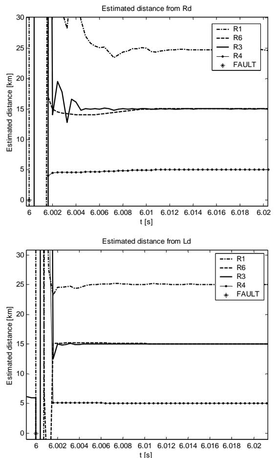
Fig. 3 estimated fault distances by  $R_1$ ,  $R_3$ ,  $R_4$  and  $R_6$  relays; a) estimate from  $R_d$ ; b) estimate from  $L_d$
