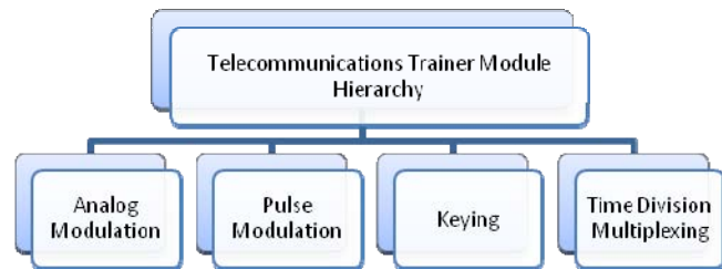
Fig. 5 The telecommunications trainer main modules
