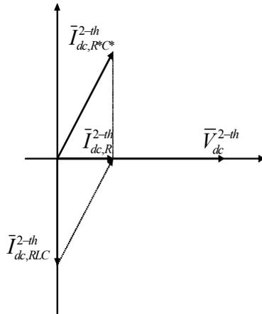
Fig. 4. Calculation of the PFC's 2-th harmonic current,  $\bar{I}_{dc,R^*C^*}^{2-th}$ , for passive PFC's parameters designing
