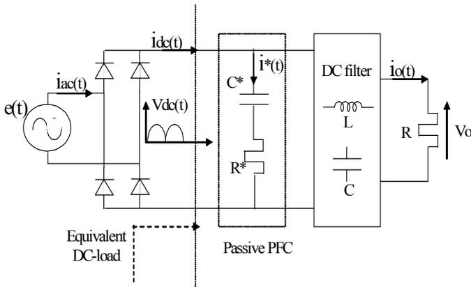
Fig. 1. Single-phase bridge diode rectifier scheme, with the introduced passive PF
