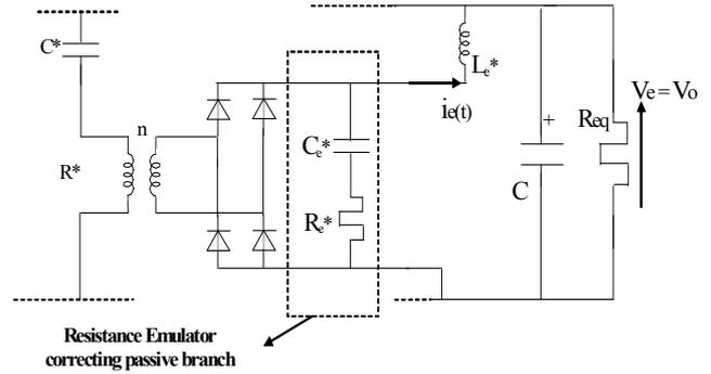
Fig. 8. Equivalent circuit of the Resistance Emulator, for its passive correction
