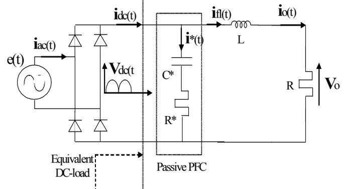
Fig. 2. Single-phase diode bridge rectifier scheme with L DC-filter and the proposed passive PFC
