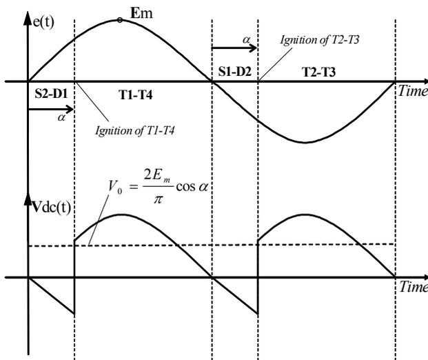
Fig. 10. Operation of the new phase-controlled rectifier switches and DC-side voltage ( $V_{dc}$ ) waveform, in presence of a fully resistive load behavior
