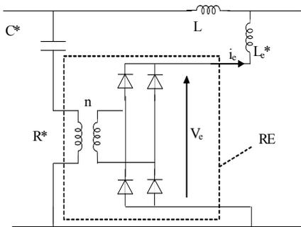
Fig. 6. The proposed resistance emulator circuit
