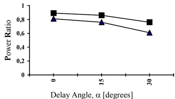
Fig. 13. Plotting the power ratio, PR, between the DC power delivered to the load and the absorbed AC apparent power, for the conventional (■) and the new (▲) rectifiers, for different values of  $\alpha$ .
