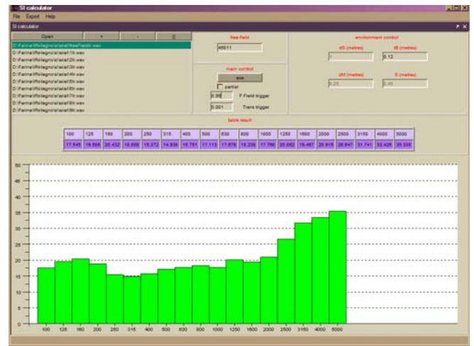
Figure 11 – Wooden barrier- Sound Insulation Index – Element - DL_{SI} = 18.5 [dB]
