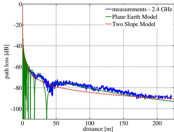
Fig. 9. Comparison of measurement results and path loss models for open area;  $f= 2.4$  GHz
