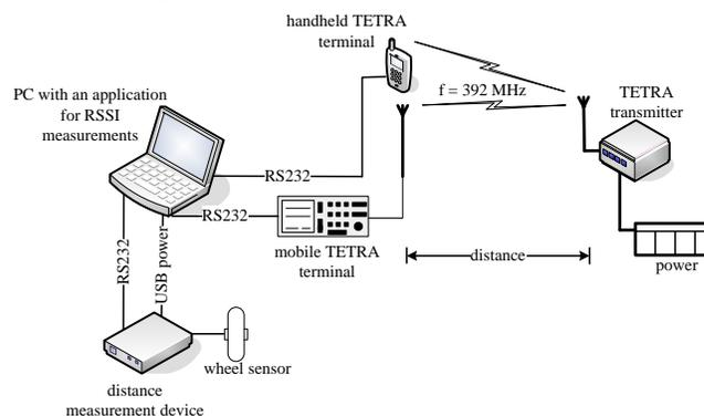
Fig. 4. Measurement setup – TETRA system
