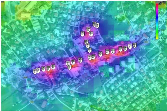
Fig. 10. Coverage of wireless sensor testbed in the city environment;  $f=868$  MHz
