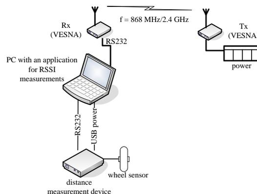
Fig. 3. Measurement setup – sensor system
