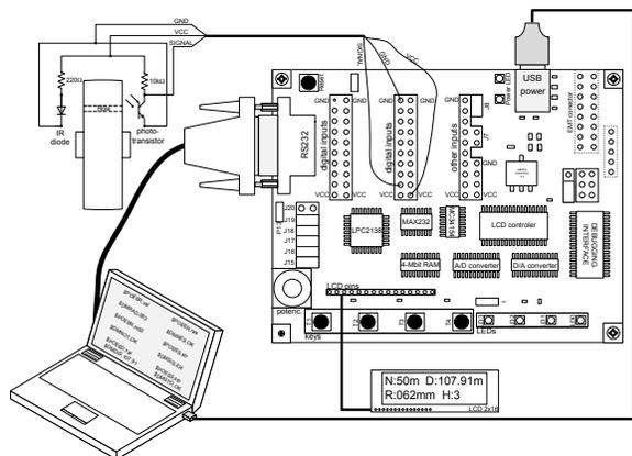
Fig. 2. Distance measurement device block scheme
