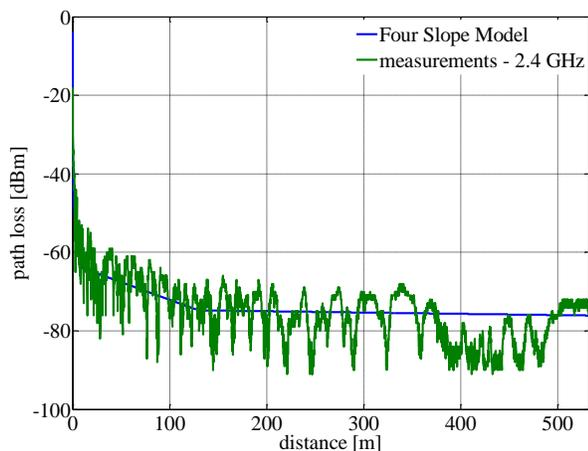
Fig. 14. Comparison of measurement results and path loss model for tunnel;  $f=$  2.4 GHz
