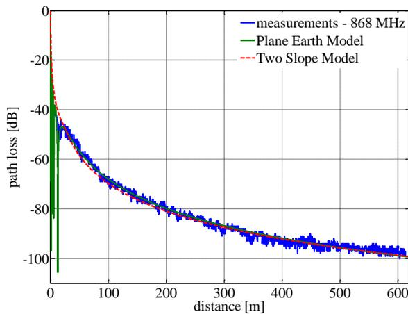
Fig. 8. Comparison of measurement results and path loss models for open area;  $f= 868$  MHz
