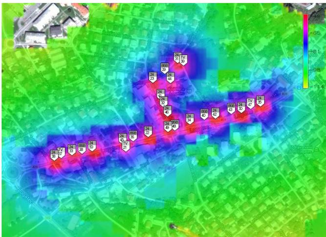
Fig. 11. Coverage of wireless sensor testbed in the city environment;  $f=2.4$  GHz
