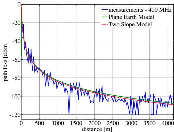
Fig. 7. Comparison of measurement results and path loss models for open area;  $f= 400$  MHz
