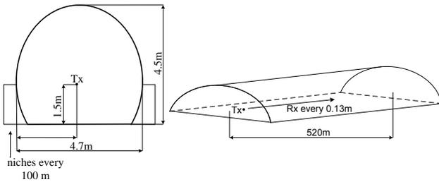
Fig. 6. Railway tunnel
