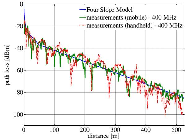
Fig. 12. Comparison of measurement results and path loss model for tunnel;  $f=400$  MHz
