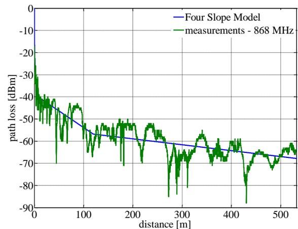
Fig. 13. Comparison of measurement results and path loss model for tunnel;  $f=868$  MHz
