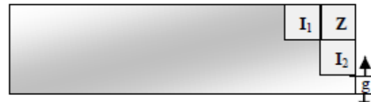
Figure 4 The encoder-aware parity check matrix structure
