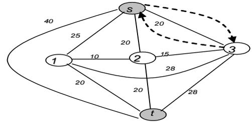
Fig. 2. A mesh network with terminal set  $K=\{s,t\}$  (each node has  $SNR=1000$ , transmission rate  $R = 1$  bit per channel use, and the fading state of each channel has expected value  $\mu=1$ ).
