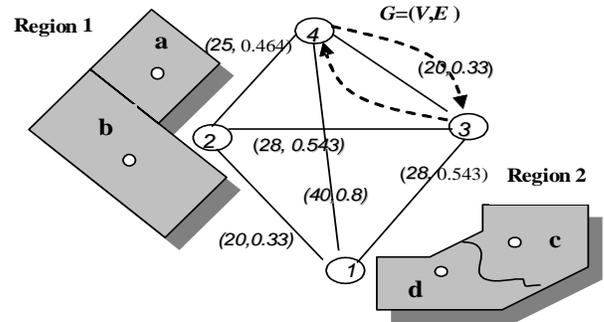
Fig. 6. Existing network  $G=(V,E)$  and regions  $\mathbf{R}_1$  and  $\mathbf{R}_2$  with corresponding areas A, B, and C, D with centroid nodes a, b, and c, d, respectively. The first value of an ordered pair represents the distance between two nodes and the second value is the probability of failure of the anti-parallel links.
