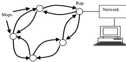
Fig. 1. An example of a mesh network modeled as a digraph.
