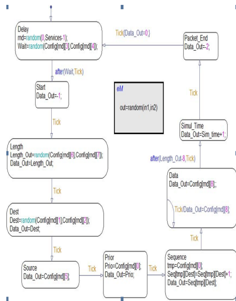
Fig. 4 Algorithm for packet generation
