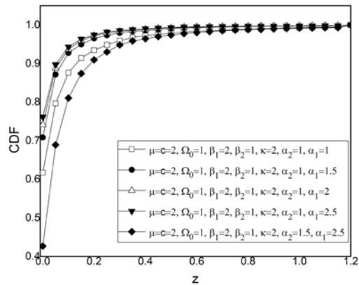
Fig. 4. CDF of macrodiversity system depending on output signal to interference ratio z
