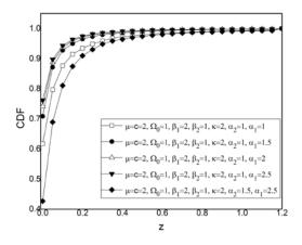
Fig. 4. CDF of macrodiversity system depending on output signal to interference ratio *z*
