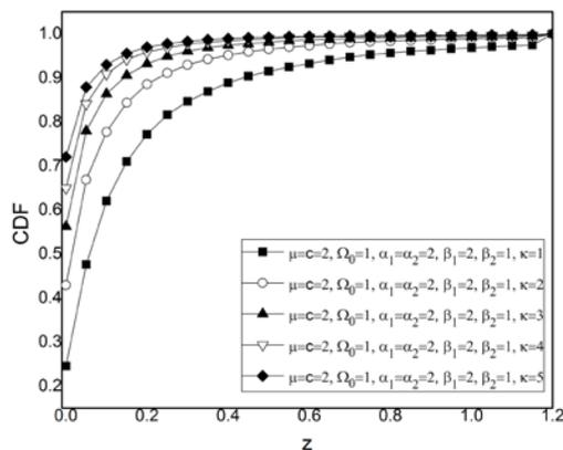
Fig. 2. Outage probability of macrodiversity system versus output signal to interference ratio
