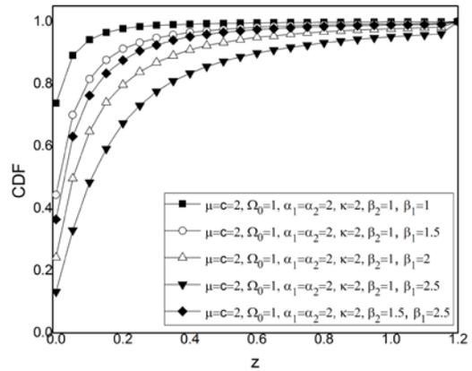
Fig. 3. CDF of macrodiversity system versus output signal to interference ratio z
