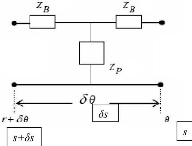
Fig. 1 Schematic of a 4-port T-circuit.
