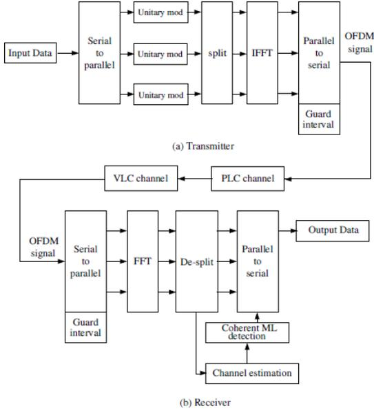
Fig. 1: Proposed PLC-VLC/UFM-OFDM system.
