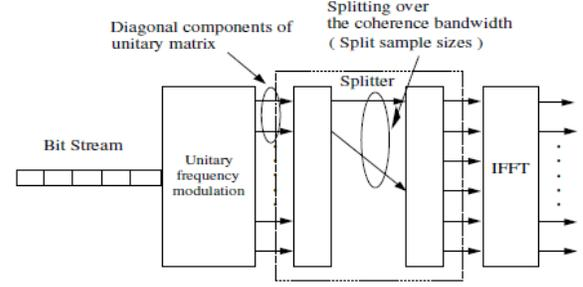
Fig. 2: Frequency splitter.
