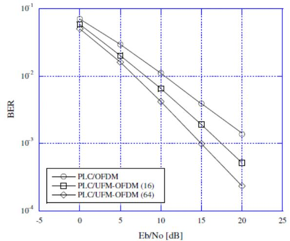
Fig. 3: BER performance of PLC/OFDM and PLC/UFM-OFDM with splitting size of 16 and 64 for power line channels heavily distributed by impulsive noise ( $A=0.001$ ,  $\Gamma=0.001$ ).
