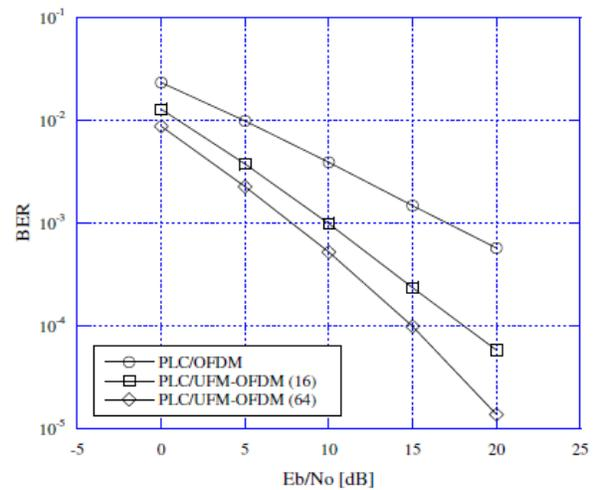
Fig. 4: BER performance of PLC/OFDM and PLC/UFM-OFDM with splitting size of 16 and 64 for power line channels weakly distributed by impulsive noise ( $A=0.01$ ,  $\Gamma=0.01$ ).
