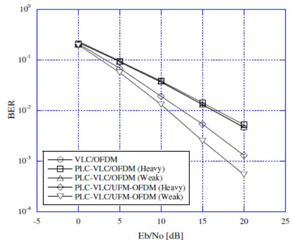
Fig. 5: BER performance of VLC/OFDM, PLC-VLC/OFDM and PLC/UFM-OFDM with heavy and weak noises.
