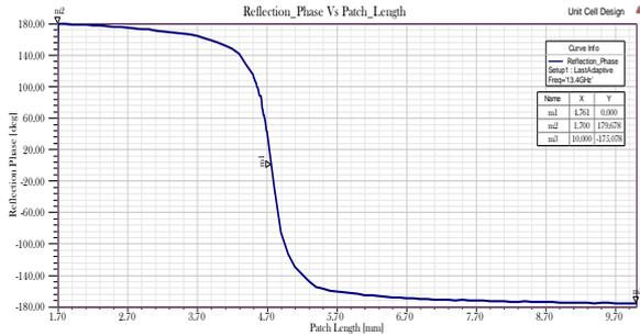
Fig 5. Reflection Phase Versus Patch Length (S - Curve)
