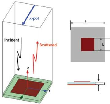
Fig 2. The infinite-array model setup of the patch element in HFSS using unit cell approach [6]
