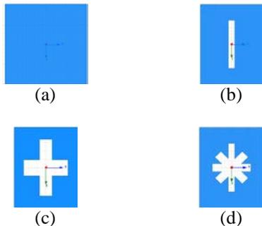
Fig 6. Different Types of Configurations In Unit Cell of Reflectarray (a) Rectangular Patch (RP) (b) Rectangular Slot (RS) (c) Plus Shape Slot (PS) (d) Star Shape Slot (SS)
