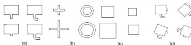
Fig 1. Various Reflectarray elements, (a) Identical patches with variable-length phase delay lines, (b) Variable-size dipoles or loops, (c) Variable-size patches, (d) Variable angular rotations.
