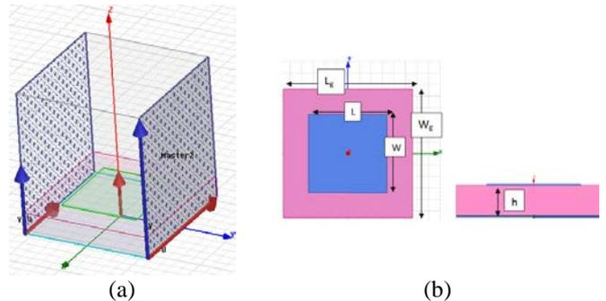
Fig 4. Reflectarray Element with (a) Master and Slave Boundary (b) Unit Cell Dimensions
