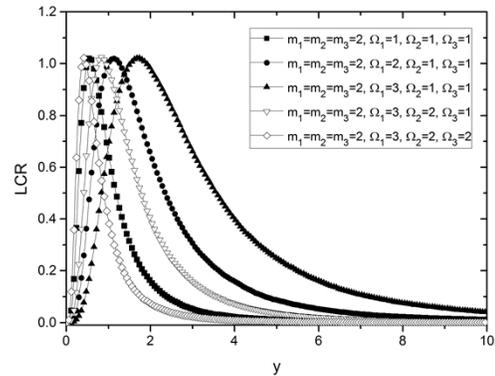
Fig. 1. LCR of the ratio of Nakagami- $m$  random process and product of two Nakagami- $m$  random processes
