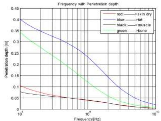
Fig. 1. The relation between frequency range(100MHz-10GHz) and penetration depth for the different tissues [3].
