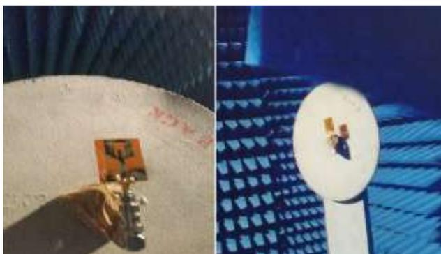
Fig. 3. Fabricated proposed antenna under measurement in Anechoic Chamber.
