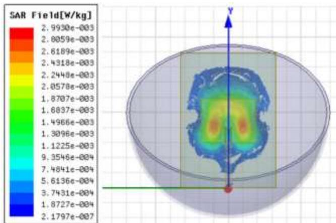
Fig. 9. SAR distribution on fatty tissue of breast phantom.
