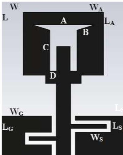
FIG. 2. The proposed flexible CPW antenna
