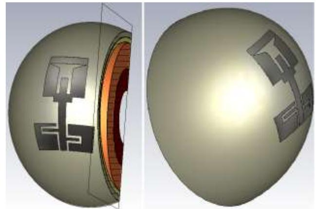
Fig. 8. The flexible antenna bended on the breast phantom.
