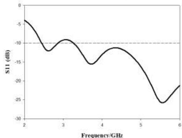
Fig. 9. S11 of the bended structure.
