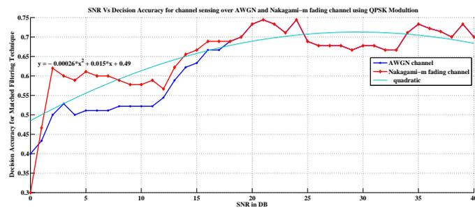
Fig. 5. Decision accuracy of Matched filtering technique over AWGN and Nakagami-m fading channel using QPSK modulation
