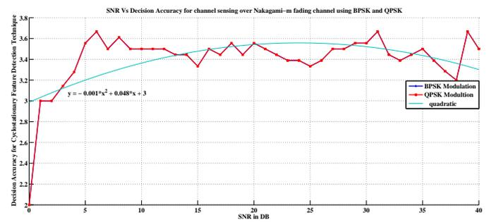
Fig. 12. Decision accuracy of Cyclostationary Feature Detection technique over Nakagami-m fading channel using BPSK and QPSK modulation
