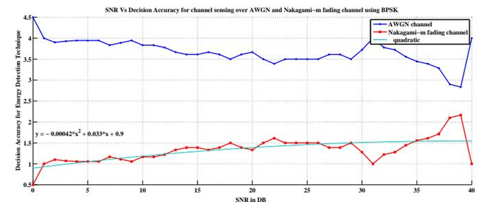
Fig. 7. Decision accuracy of Energy Detection technique over AWGN and Nakagami-m fading channel using BPSK modulation
