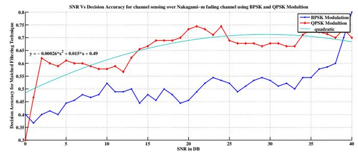
Fig. 6. Decision accuracy of Matched filtering technique over Nakagami-m fading channel using BPSK and QPSK modulation
