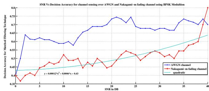
Fig. 4. Decision accuracy of Matched filtering technique over AWGN and Nakagami-m fading channel using BPSK modulation
