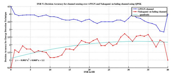
Fig. 8. Decision accuracy of Energy Detection technique over AWGN and Nakagami-m fading channel using QPSK modulation
