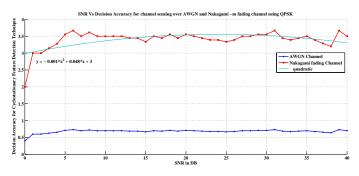
Fig. 11. Decision accuracy of Cyclostationary Feature Detection technique over AWGN and Nakagami-m fading channel using QPSK modulation
