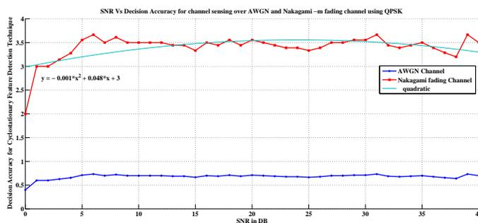
Fig. 11. Decision accuracy of Cyclostationary Feature Detection technique over AWGN and Nakagami-m fading channel using QPSK modulation
