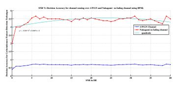
Fig. 10. Decision accuracy of Cyclostationary Feature Detection technique over AWGN and Nakagami-m fading channel using BPSK modulation
