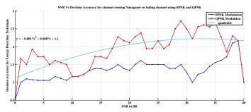
Fig. 9. Decision accuracy of Energy Detection technique over Nakagami-m fading channel using BPSK and QPSK modulation
