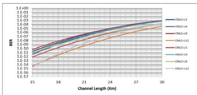
Fig. 11 BER vs channel length
