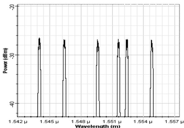
Fig. 4 First user spectrum showing the code weight is 6
