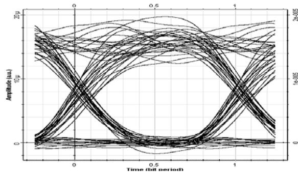
Fig. 7 Eye pattern of the first user after balanced detection
