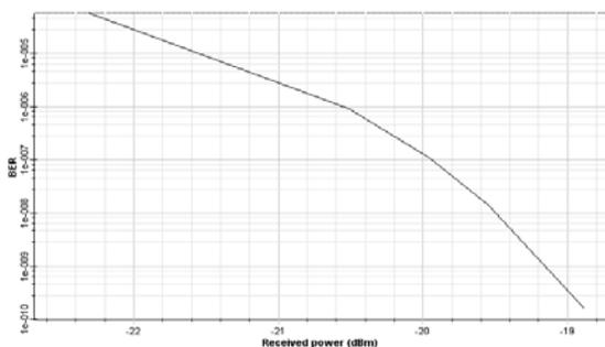
Fig. 16 Eavesdropper BER versus measured receiver sensitivity
