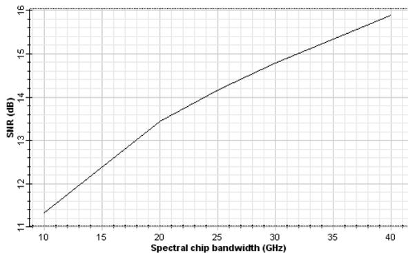
Fig. 15 Influence of the spectral chips bandwidth on the eavesdropper SNR
