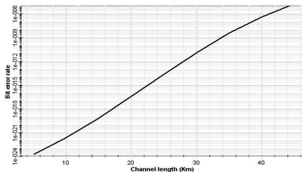
Fig. 8 BER vs channel length
