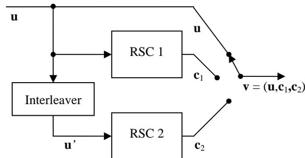
Fig. 1. The turbo encoder with rate 1/3.
