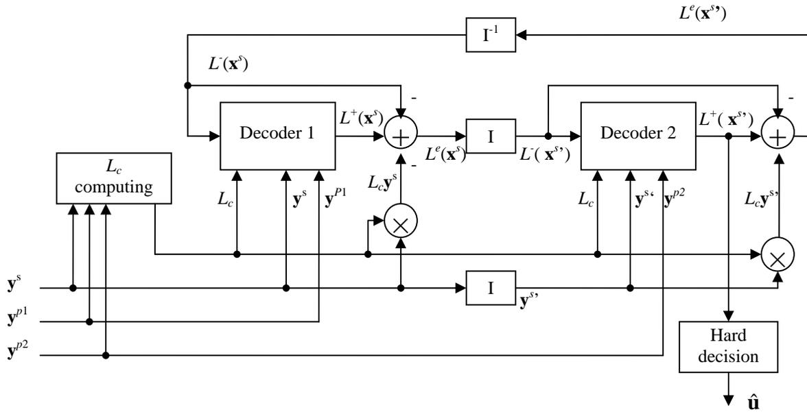
Fig. 2. The turbo decoder.
