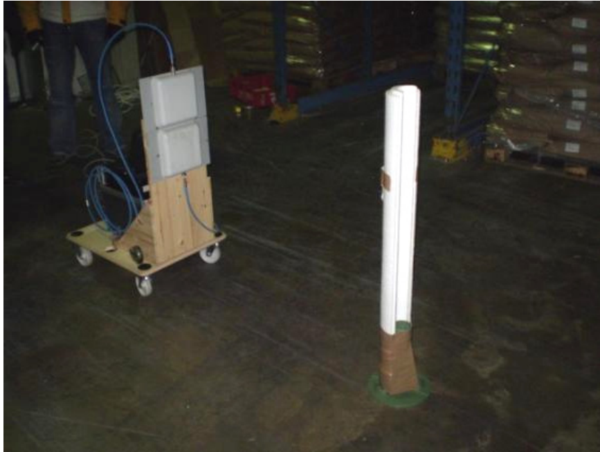
Fig.3. The test set-up for Gen2 tag measurements in cold conditions
