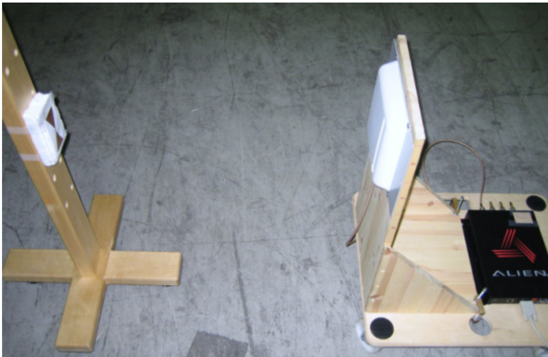
Fig.1. The test set-up for Gen1 tag measurements
