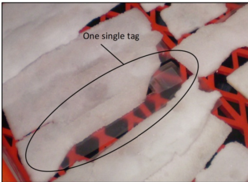
Fig.4. The Gen2 tags covered with ice
