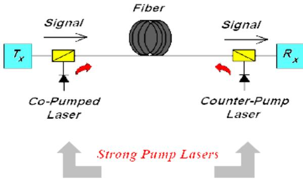
Fig. 1 Schematic of a DRA used in optical communication system
