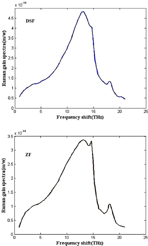
Fig.8 The Raman gain spectrum for dispersion-shifted Fiber (DSF) and Z-fiber
