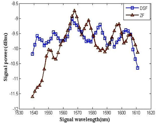
Fig.9 Signal powers for DSF and ZF
