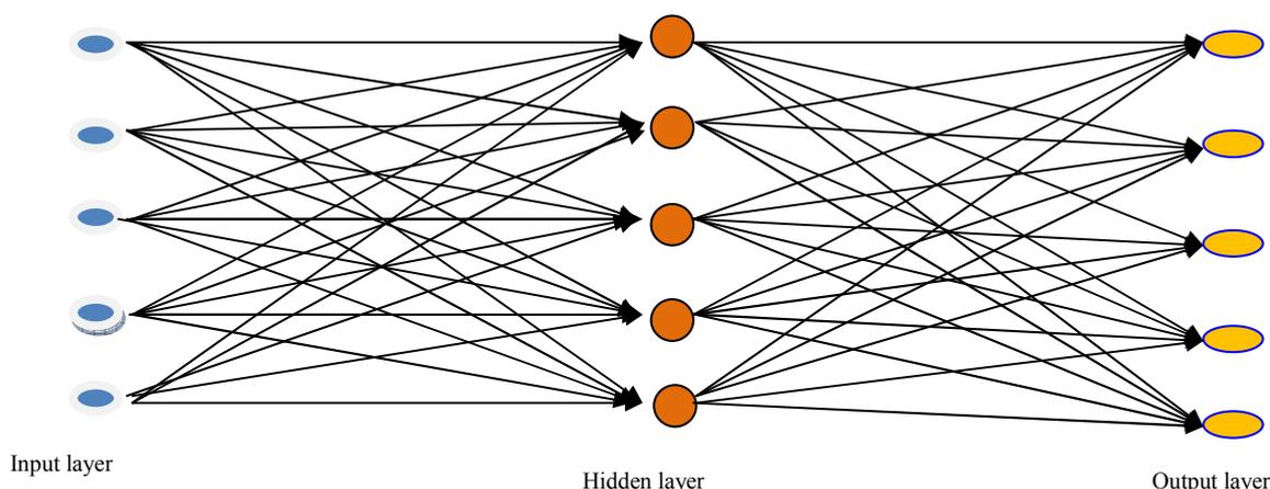
Figure 4. The Artificial Neural Network in the Multi Layer Perceptron topology of 5 neurons per layer
