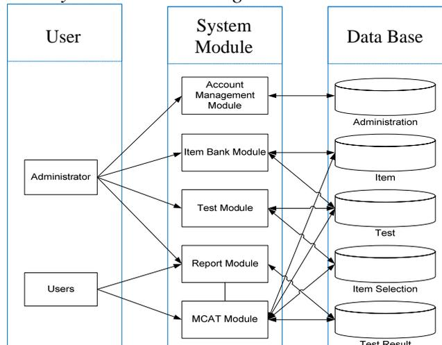
Figure 5. MIRT Based MCAT modular Structure
