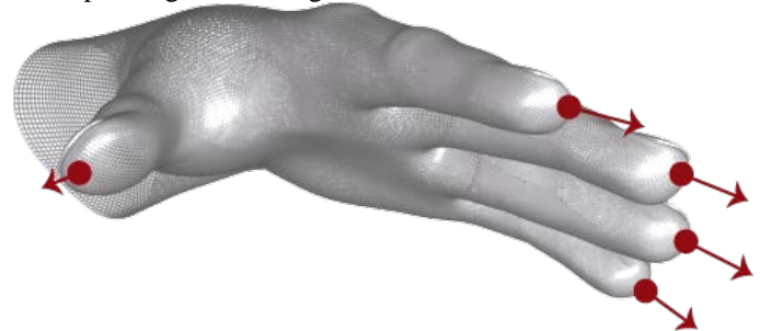
Fig 3 The direction is expressed as a unit vector pointing in the same direction as the tip, from [9] citation
