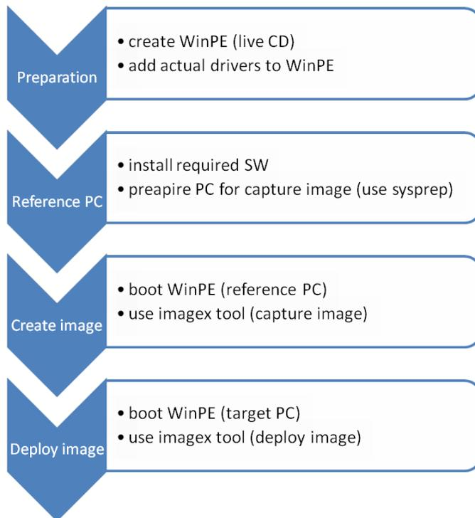
Fig. 1 Phases of automated unattended installation
