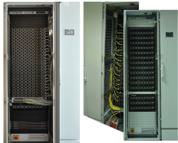
Fig. 4. RCS based on Xilinx Virtex-7 FPGAs (a – RCS-7 on the base of the CM Pleiad, b – RCS on the base of the CM Taygeta)
