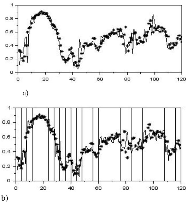
Fig.1. Original line (dotted curve) and its reconstructed (continuous curve); a) the regular stationary segmentation, b) the irregular stationary segmentation, where the vertical lines delimit the stationary segments.
