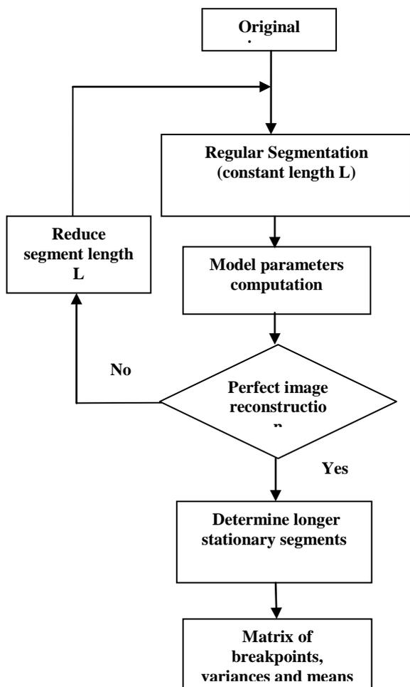
Fig. 2. The image irregular compression algorithm.
