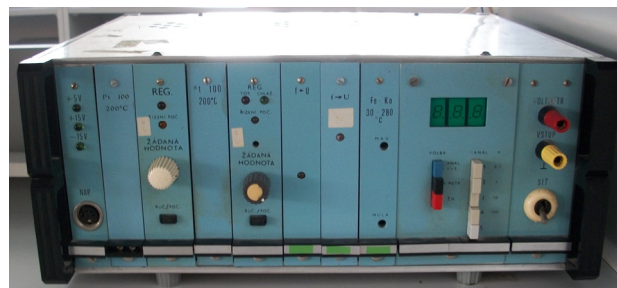
Fig. 1 the appearance of the former obsolete I/O converter and control unit
