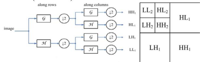
Fig. 4. DWT decomposition scheme
