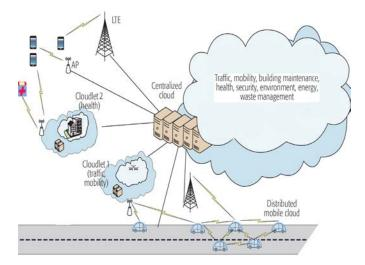
Fig. 2 Cloud topologies in a unified urban mobile computing offloading mechanism [7].
