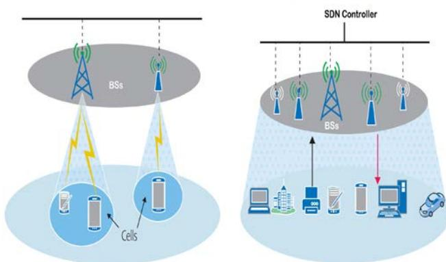
Fig. 4 Conventional cellular network and cell-less network [2].
