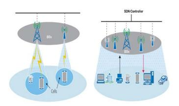
Fig. 4 Conventional cellular network and cell-less network [2].
