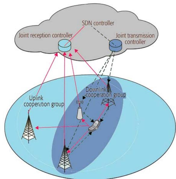
Fig. 5 Transmission model of a cell-less network [2].
