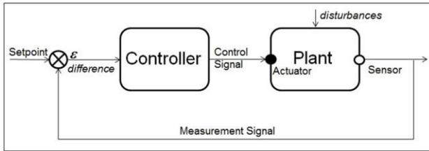
Fig. 1. Feedback control system principle.
