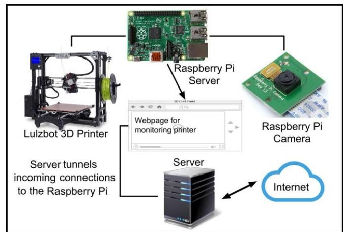
Fig. 5. Physical diagram of 3D printer connectivity.
