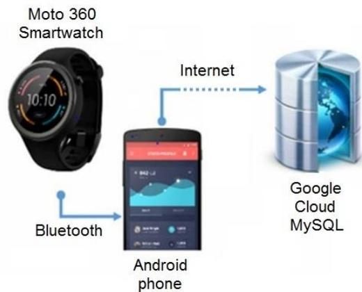
Fig. 10. Connectivity of the smartwatch with Android and cloud.
