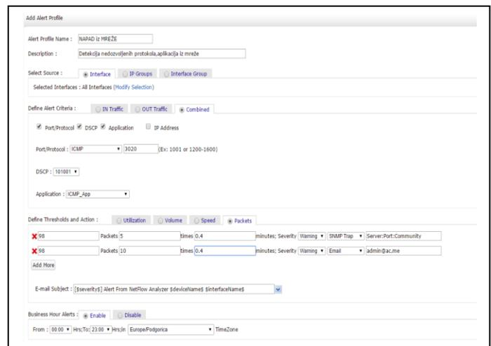
Fig. 11. Sending SNMP Trap alert messages for the ICMP protocol, DSCP-101001 and ICMP application
