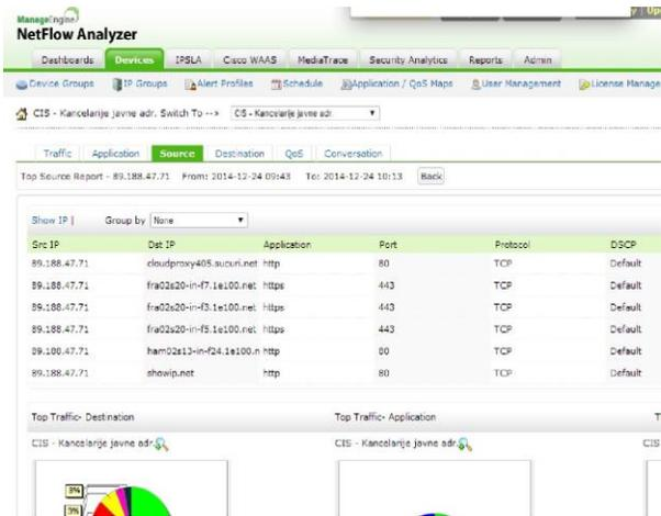
Figure 1. An overview of the connections executed by a specific host with a depicted DNS
