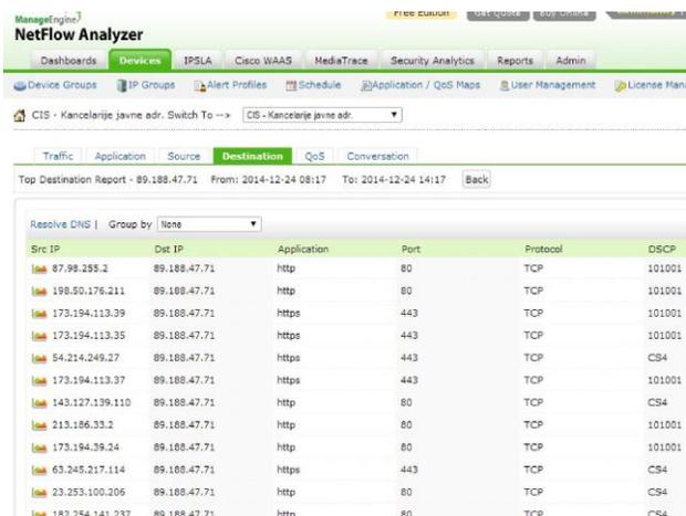
Figure 2. An overview of the connections executed by a specific host without a depicted DNS
