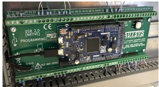
Fig.7 PCB with socket for Arduino
