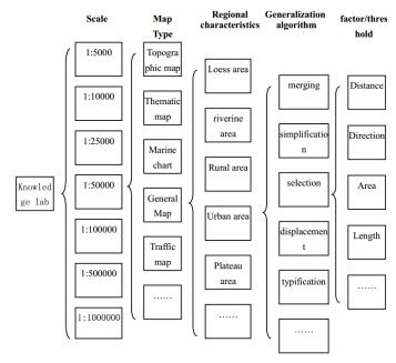
Fig. 3 the structure of generalization knowledge lab shown as fig 6.4. Firstly, knowledge is classed by scale, map type, regional characteristic. Secondly, it is divided by generalization algorithm. And finally, the factor and threshold is decided by actual generalization scenes and algorithm characteristic.
