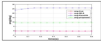
Fig. 7. Voltage angle at bus 13 Comparison between WLS, Kaushik Das, proposed results and True values
