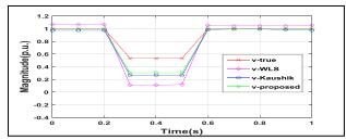
**Fig. 8**. Voltage magnitude for bus 7 at a three phase fault on bus 7
