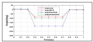
Fig. 9. Voltage angle for bus 7 at a three phase fault on bus 7
