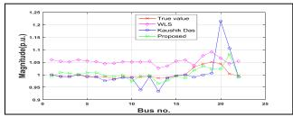
Fig. 4. Voltage Magnitude Comparison between WLS, Kaushik Das, proposed results and True values.
