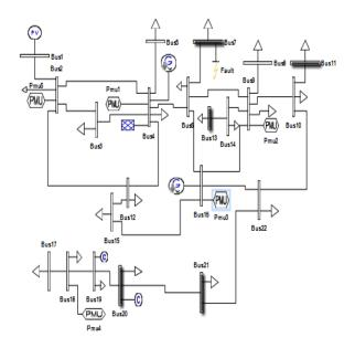
Fig. 3. 22-Bus Alexandria Network 220Kv Transmission System
