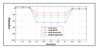
Fig. 11. Voltage angle of bus 6 for a three phase fault on bus 7
