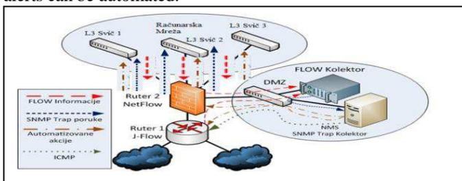
Figure. 9. Elements of control systems - Connecting switches, Flow collector
