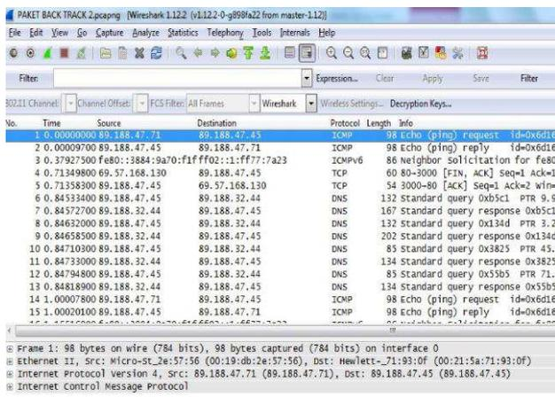
Figure 4. Intercepted packets from all IP addresses in the network, without the use of filters
