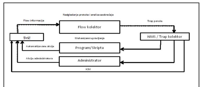
Figure. 10. Schematic representation of management process
