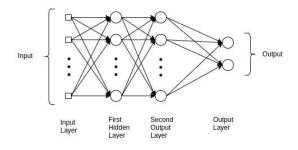
Fig. 3. 3-layer multilayer perceptron model [10]
