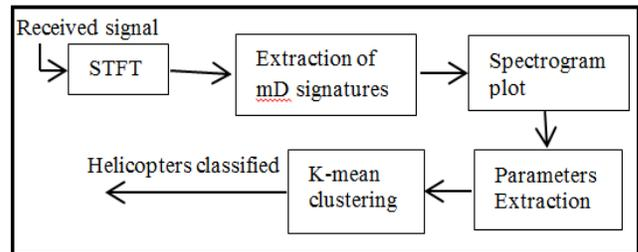
Fig.4. Block diagram representation of mD extraction and helicopter classification process
