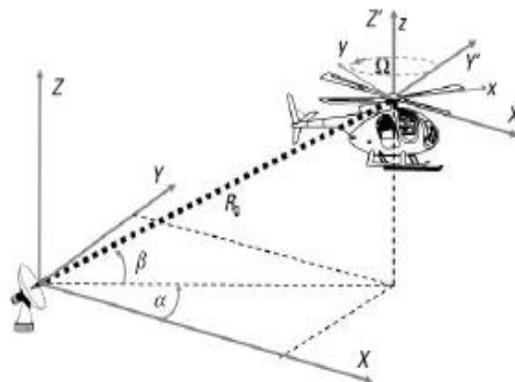
Fig.1. Geometry of RADAR (courtesy V. C. Chen [1])
