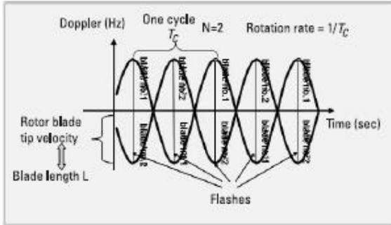
Fig.5. Micro-Doppler signature of a rotor with 2 blades (courtesy V. C. Chen [1])
