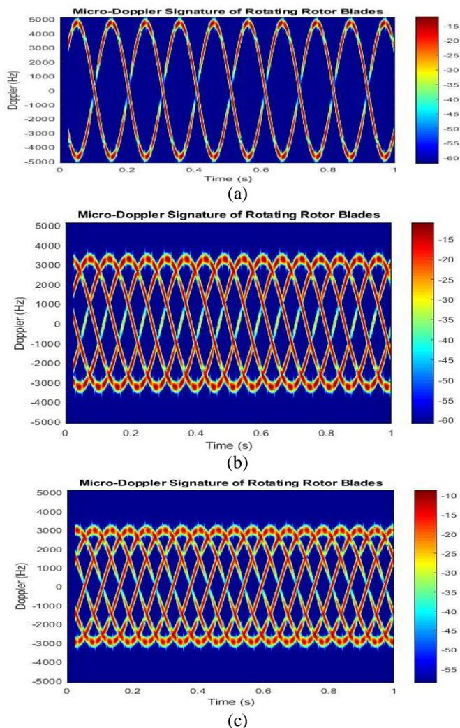
Fig.7. Spectrograms of 3 different helicopters of interest. (a) Spectrogram of the helicopter UN-1N (rotor with 2 blades). (b) Spectrogram of the helicopter SH-3H (rotor with 5 blades). (c) Spectrogram of the helicopter CH-54B (rotor with 6 blades).
