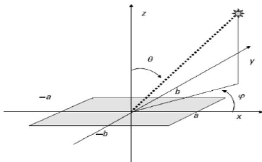
Fig.3. Rectangular flat plate modelled as the rotor blade (courtesy V. C. Chen [1])
