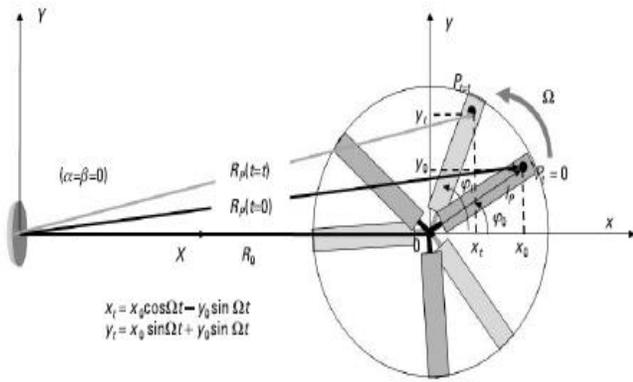
Fig.2. Rotation of rotor blades (courtesy V. C. Chen[1])
