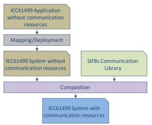
Fig. 5. IEC61499 system development with composition.
