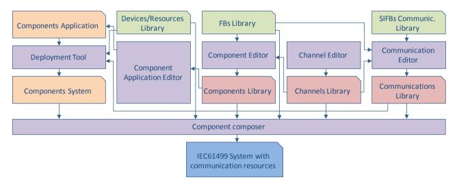
Fig. 7. IEC61499 system development with components, translate and composition.
