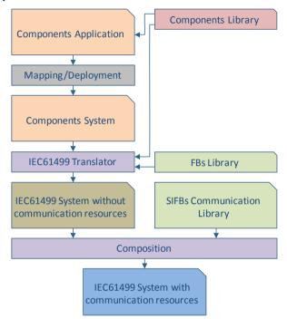
Fig. 6. IEC61499 system development with components, translate and composition.
